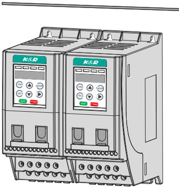
Installing drive side by side
